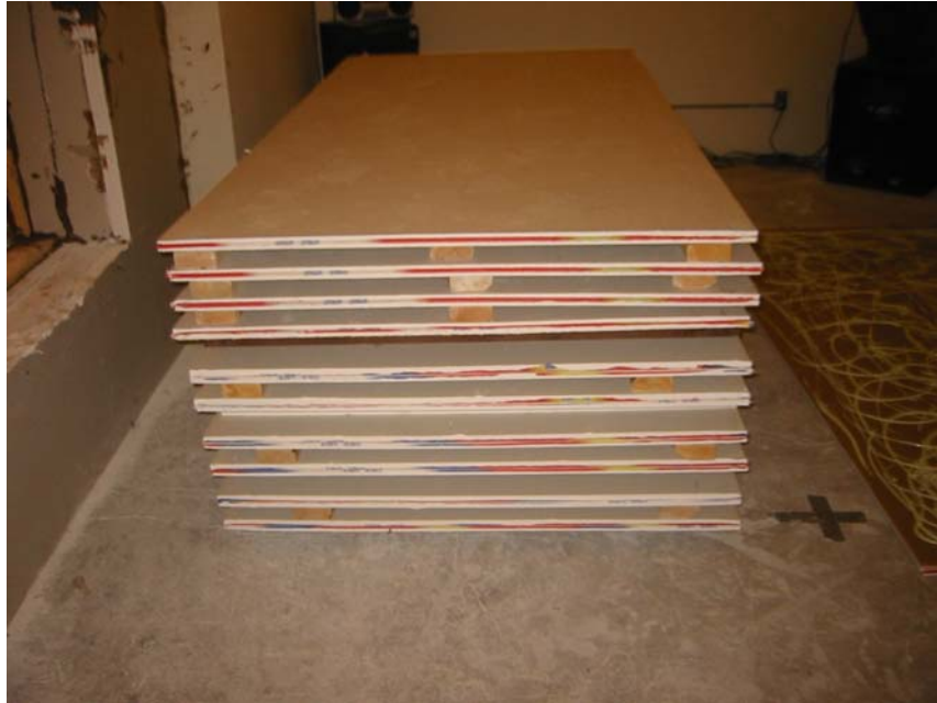
Figure 2: Pre-constructed sandwich panels stacked and spaced for drying.
