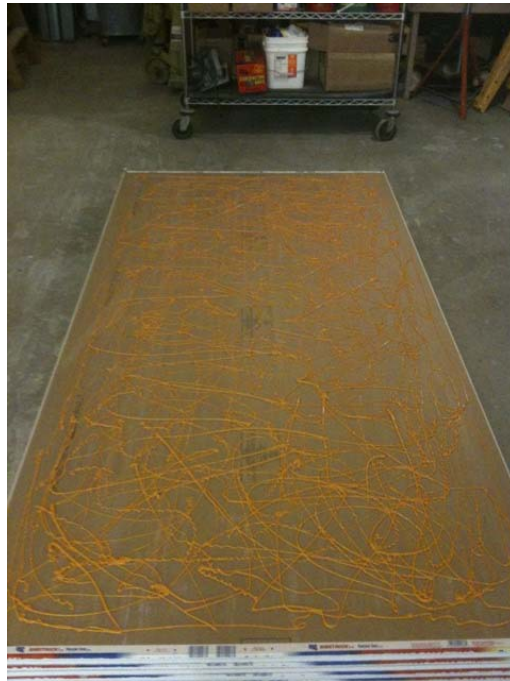
Figure 1: Representative damping adhesive application prior to adding 2 nd layer of sheeting to sandwich.
